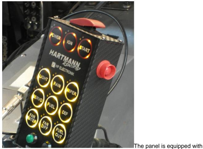
12 buttons, each button has two functions - Momentary and Toggle. - NEW! Now you have also a possibility to make 2 stages on your output, first push A next B third off, or/and A, A+B and off. Also we are now supporting Can speed 500Kbit and 1Mbit - Please see Technical Manual V.2 -
